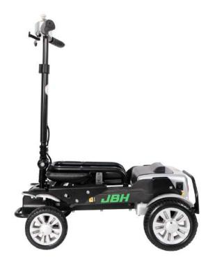
**Battery position** Under the seat of scooter
